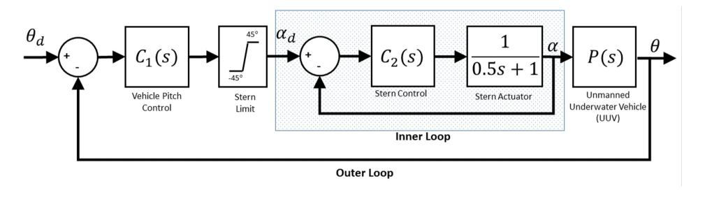
In this example an inner-loop controller is used to control the pitch of the stern plane. An outer-loop PD controller is used to control the pitch of the vehicle and feeds into the inner loop.
