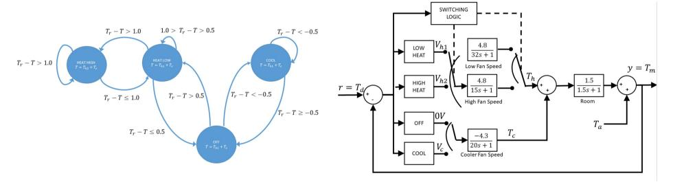
In this example we take the heating and cooling example a little further by introducing a more complex system where the system has a heater, cooler, and variable speed fan. The different elements of the system require different control strategies and even actuators, and thus hybrid control is a perfect fit.
